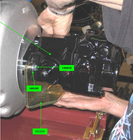
Place MNT-FWD/REV DSL SW/62 PLTD under PUMP-MAIN VD FS, as shown above. Insert screws with washers through mount into holes in bell housing. Tighten.
