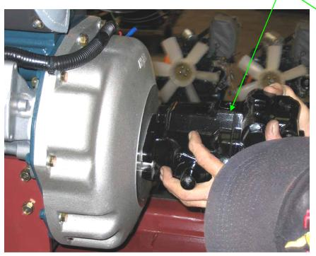
Get (1) PUMP-MAIN VD FS (**3303581**) and insert shaft into splines of flywheel at center of bell housing, as shown. Get (1) MNT-FWD/REV DSL SW/62 PLTD (**3312231**), (2) SCRS-HEX,3/8-16X1.50 ZP (**3400028**) and (2) WASHERS-CONICAL SPRING 3/8 (**3400385**).
