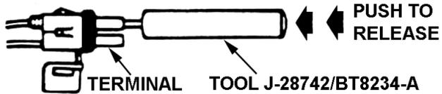
2. Remove terminal using tool.
