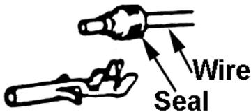
3. Cut wire immediately behind cable seal
