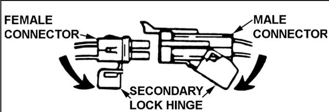
1. Open secondary lock hinge on connector.
