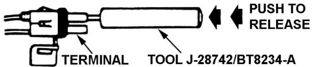
2. Remove terminal using tool.
