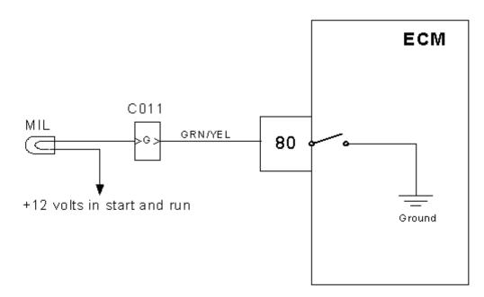
OBD System Check/ MIL (Malfunction Indicator Lamp)
