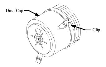
The dust cap should be removed and cleaned on a 8 hour basis.
