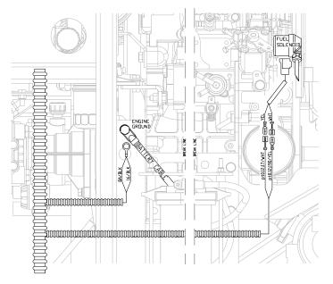
**Engine Ground and Fuel Solenoid Connections**
