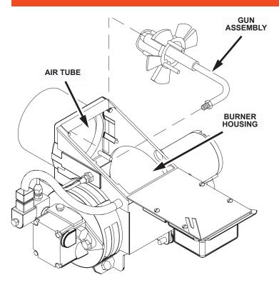
NOTE: The Gun adjustment guide is set at position 4, leave adjustment guide in this position.
