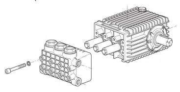
NOTE: It may be necessary to tap head lightly with mallet to loosen.
