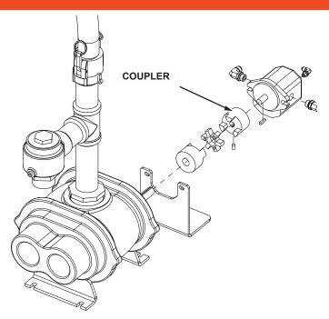
10. Slide the new motor on to the coupler attached to the roots blower and secure the new motor with the 2 screws, washers, and locking nuts,
