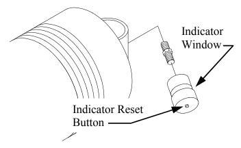
Note: The indicator may return to the non-visible position when the engine is shut off. To check, reset indicator and turn on engine, if it locks in visible position again, notify maintenance department to change filter.
