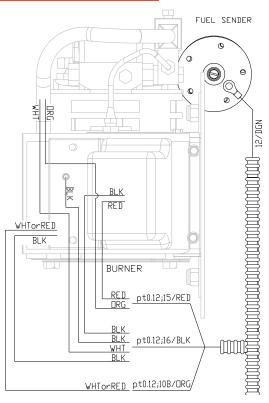
**Alternator and Burner Thermostat Connections**
