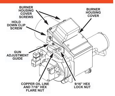
8. Install new gun assembly into the burner housing, grasp the gun assembly from the oil line fitting. Holding the gun assembly at a 45° angle gently slide the nozzle into the housing and the air tube
