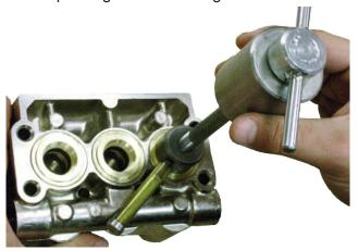
8. Place proper insertion tool in cylinder and install front head ring, v-packing and long life ring and press firmly into cylinder until they will go no further using proper insertion tool.
