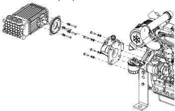
19. Remove gear reducer and water pump together, Remove 4 screws, lock and flat
