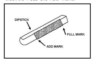
Figure 2 Engine Oil Dip tick (Typical)
