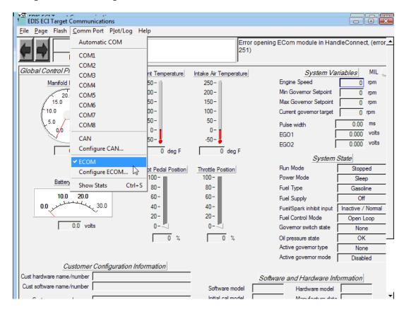
To connect using the ECOM cable you must select ECOM from the COM Port drop down menu.
